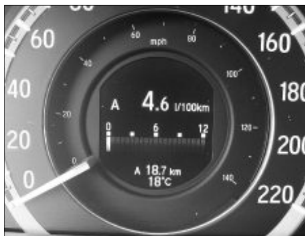
The driver information centre set in the speedometer displays several functions, such as average fuel consumption.
