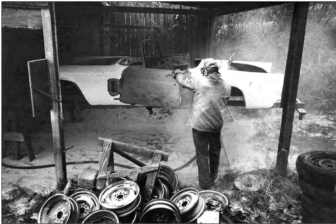
The body of the 1956 Thunderbird was taken to Snohomish, Washington for sandblasting during the complete restoration in the 1970s.
