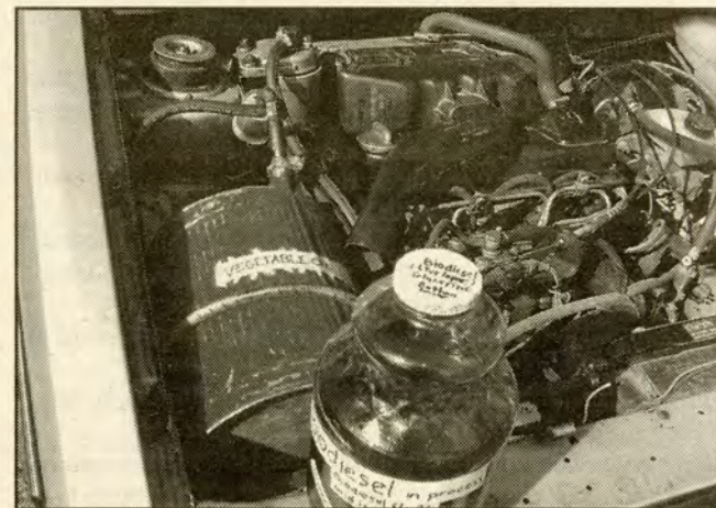
UNDER THE HOOD: A tank to hold vegetable oil has been added to the Rabbit's inner workings. No modifications are required to run the car on biodiesel.
