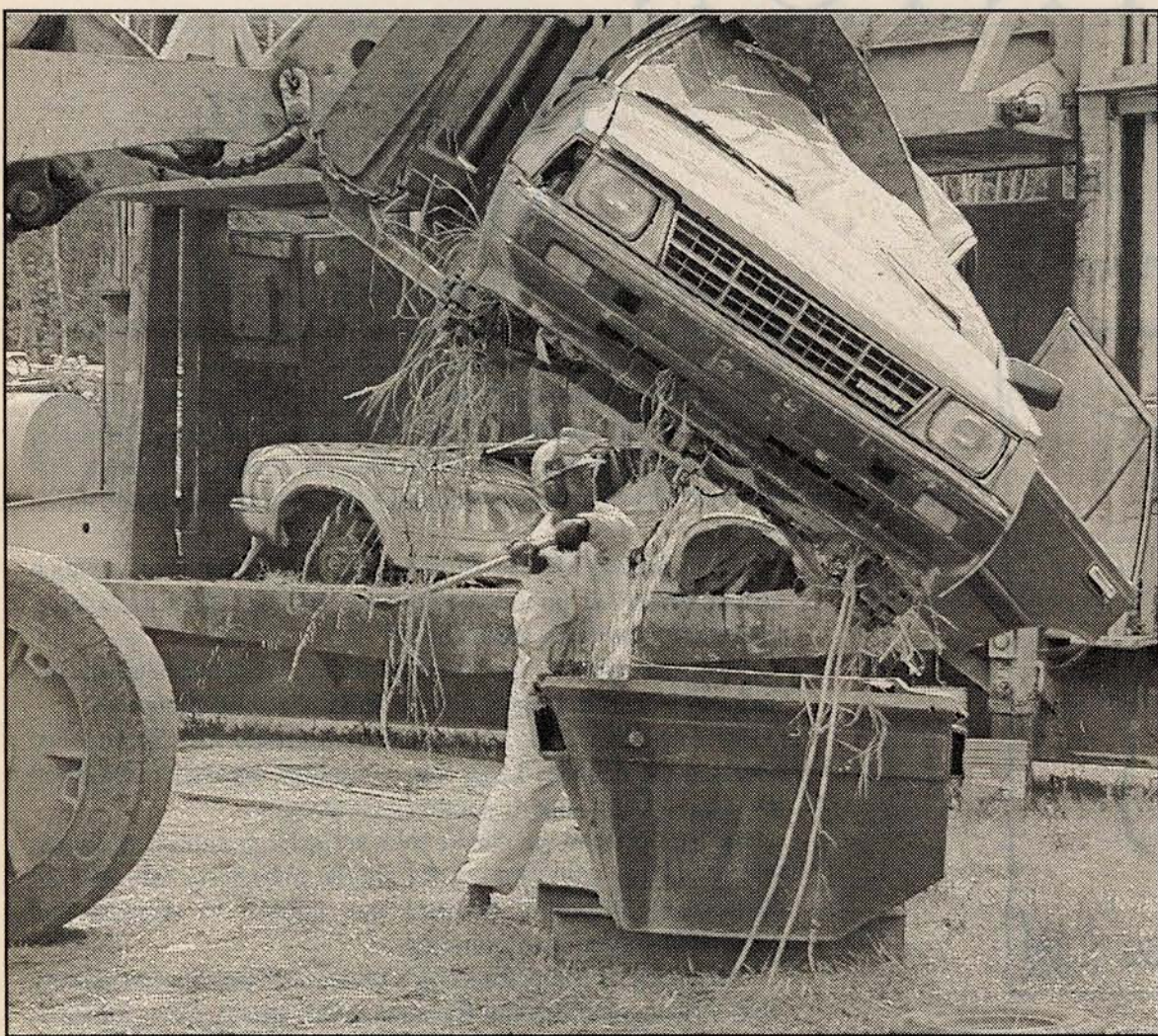
CAR CRUSHER: The Budget Steel boys and Auto Repairs. here the worker removes gas from a vehicle before it meets its doom.
