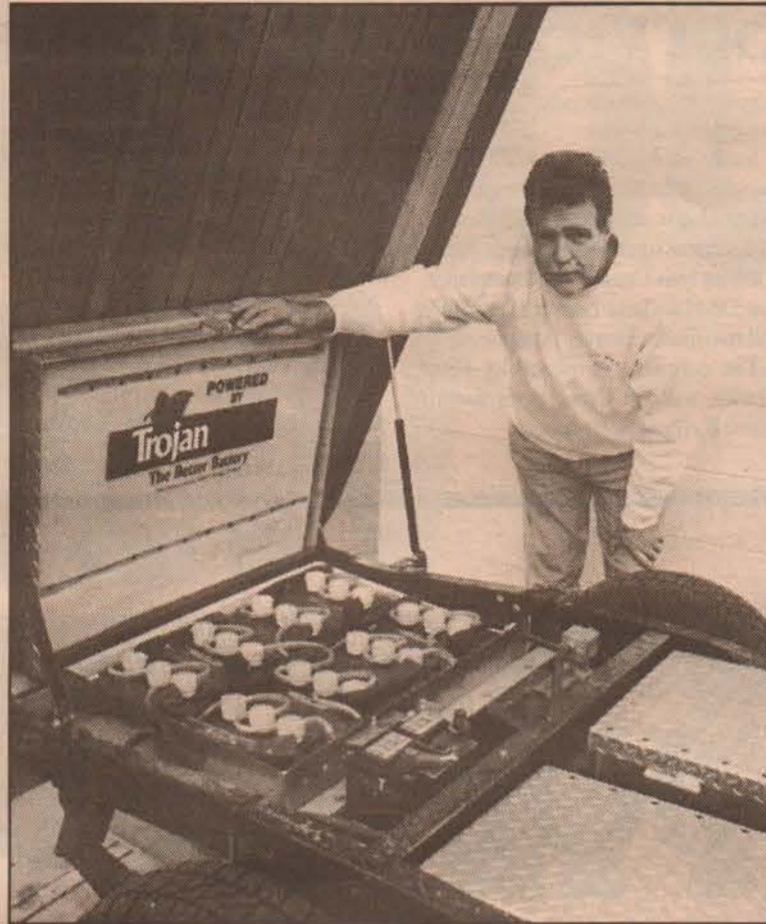
BATTERIES INCLUDED: Geoff Barrett shows the location of the battery storage compartments underneath the flat deck of the 1987 Nissan, converted to electric power.
