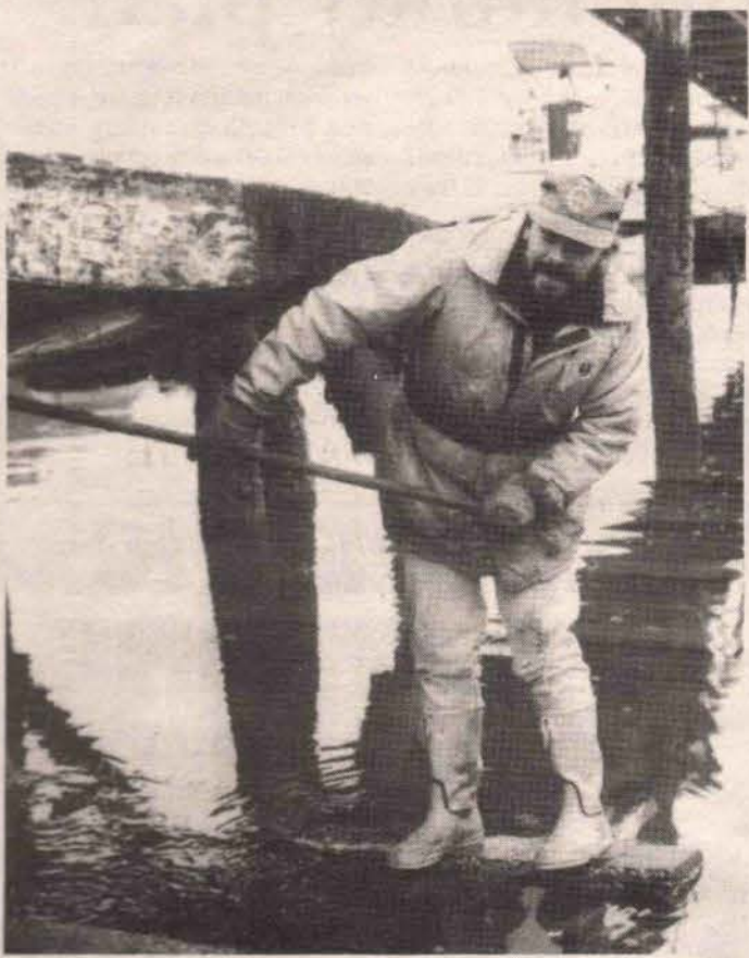
SCOURING THE BOTTOM: Robert Lavoie, skipper of the 26-foot Force Five , is cleaning off more than a year's growth of seaweed. The unwanted greenery acts as a drag under sail — so off it goes!
