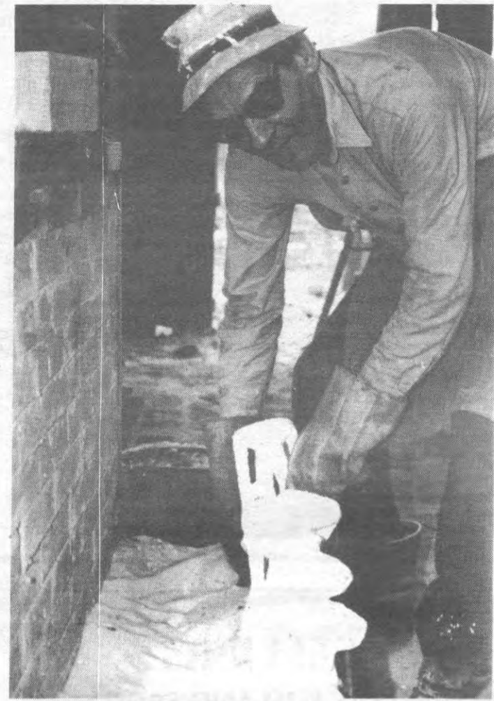
FIRED UP: Salt Spring Islander Mel Marchbank, of the Phoenix Art Foundry on Musgrave Road, places ceramic shell from kiln in sand. Marchbank is one of the only people in the province using the ceramic shell method to create bronzed artwork.
