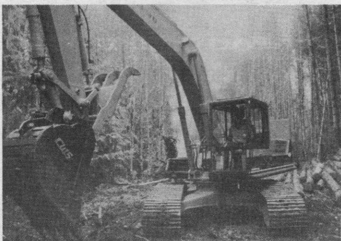
New Komatsu 1-yd. Excavator with Hydraulic Thumb
