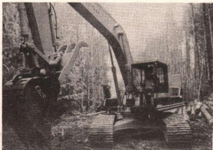
New Komatsu 1-yd. Excavator with Hydraulic Thumb
