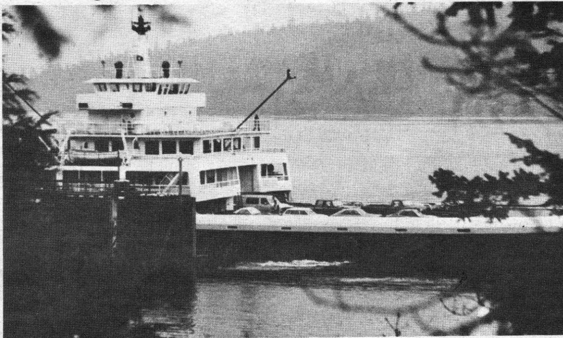
The long snout of the Bowen Queen is nosing out of Fulford dock in this picture. Lengthened ferry now matches the Mayne Queen , on the Outer Islands run. The deck, at each end of the superstructure, resembles a football field. The ships will now accommodate about 76 cars. Stretching project cost close to $5 million.
