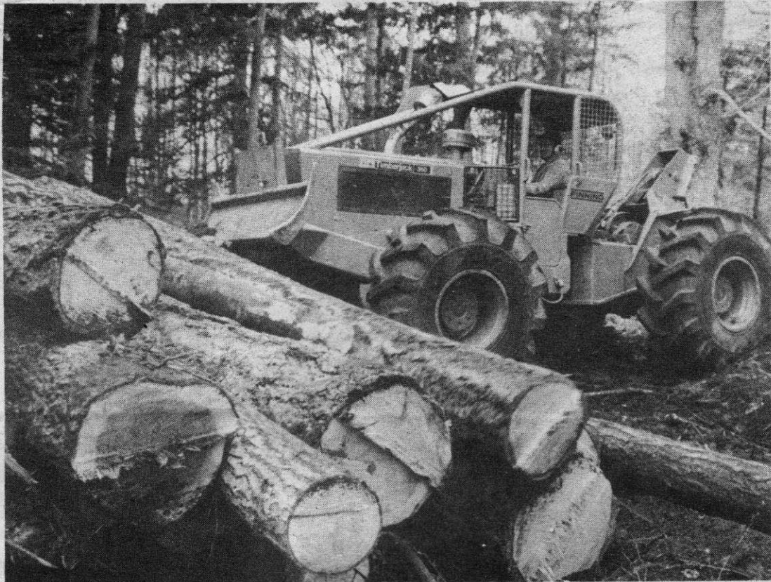
New Skidder makes work a lot less complicated for Dennis Howard [pictured] and his brother Fred of Salt Spring Island. The brothers have recently purchased the new machine, manufactured by Finning, to help with hauling and piling of timber in their logging operations.
