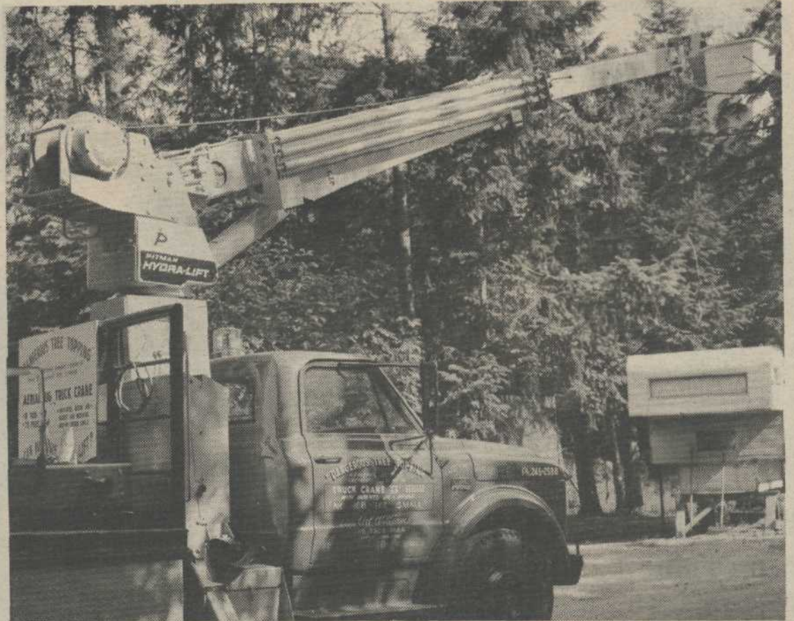
This is the new aerial rig truck crane belonging to Art Williams of Ladysmith. The bucket will extend to a height of 80 feet. Williams has been topping trees on
